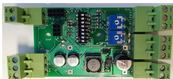
Fig. 8. Location of microswitches in the PCB EC module.
