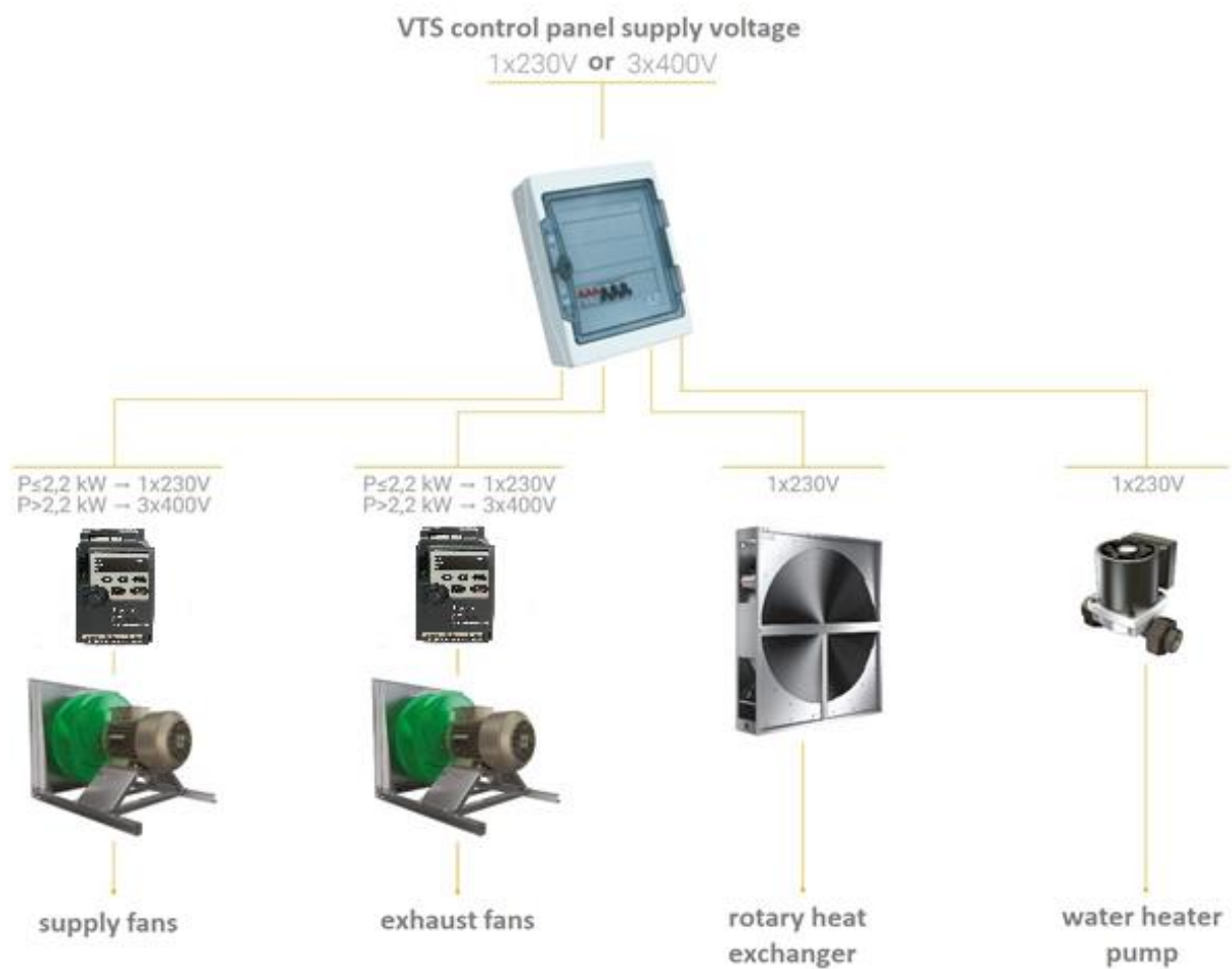
Fig. 1a Components supplied from the control panel (AHU with AC motors)
