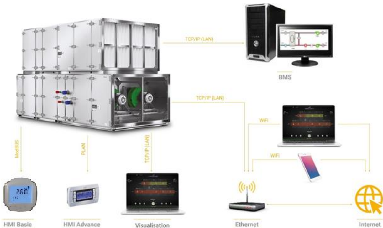
Fig. 13. Operating options of the VENTUS AHU controller.
